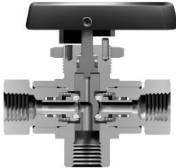
Figure 1: HB Series Ball Valve Cross Sectional View
